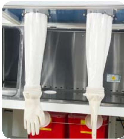
The front visor opens up fully for maintenance access into the work zone.
